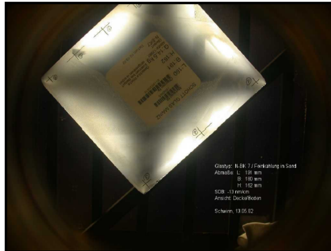
Figure 8: N-BK7 block with internal stress.
